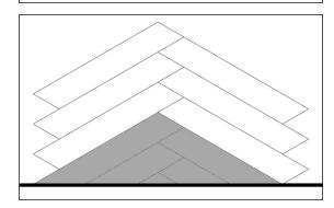
4. Repeat steps 2&3 outward the full length of the edge chosen as shown. Subsequent sets should interlock into existing sets as shown in diagram.
