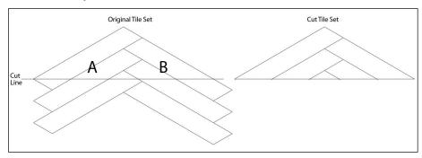
2. Once the surface is ready for the tile to be applied (follow standard instructions for installing stone tile), determine a horizontal line (often the base or edge of the install surface). Place the "cut tile set" on the edge as shown.
