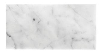
Variation in color, shade, finish, hardness, strength and slip resistance is inherent in Natural stone products. White marbles contain naturally occurring deposits of iron which may lead to discoloration of marble and turning it yellow-rust or grey if used in wet areas. This a natural characteristics of the stone and that is why it cannot be considered as a defect
