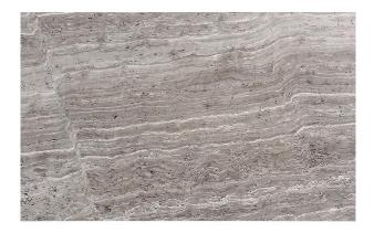
Variation in color, shade, finish, hardness, strength and slip resistance is inherent in Natural stone products. White marbles contain naturally occurring deposits of iron which may lead to discoloration of marble and turning it yellow-rust or grey if used in wet areas. This a natural characteristics of the stone and that is why it cannot be considered as a defect
